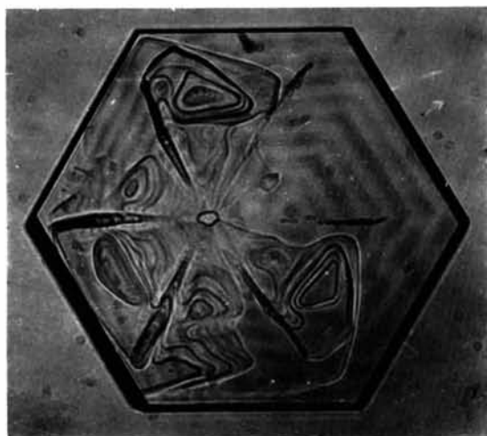
Fig. 2. Combined micrograph interferogram of crystal no. 2; (0001) face; Hg-green light ( \times 205 ).
