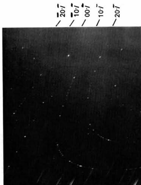
Fig. 9. Zero layer a -axis Weissenberg photograph of polytype 42R; Cu K\alpha radiation; camera diameter 5.73 cm; the festoons corresponding to 10.l and \bar{1}0.l rows of spots are recorded on the right and left side, respectively, of the straight row of 00.l spots; The first intense spot from the top corresponds to l=146 in the 10.l festoon and to l=148 in the \bar{1}0.l festoon.
